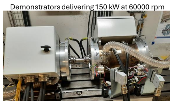
Figure 6: Back-to-back test to evaluate the performances and thermal behavior of the high-speed motors
