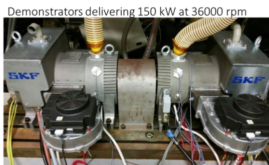
Figure 6: Back-to-back test to evaluate the performances and thermal behavior of the high-speed motors
