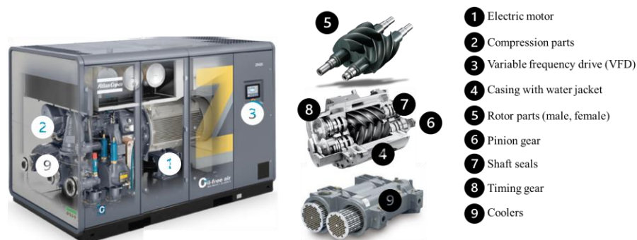
Figure 2: Illustration of a two stage WC oil-free screw air compressor with VFD (ACU from Atlas Copco)
